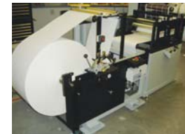
40" diameter large roll unwind, with end of roll shutoff, splice table, dancer roll, and web guide.
