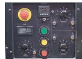
Operator control panel with programmable counter.
