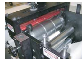
Two fully supported die stations with dual sided die frames.
